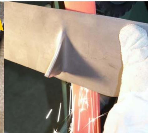
Grinding of titanium turbine blades
